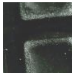
Figure 2b. Ablation resulting in an etched surface.
