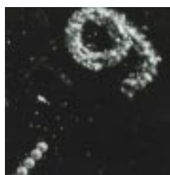
Figure 2a. Foaming of polymer to create a light image on a dark background.
