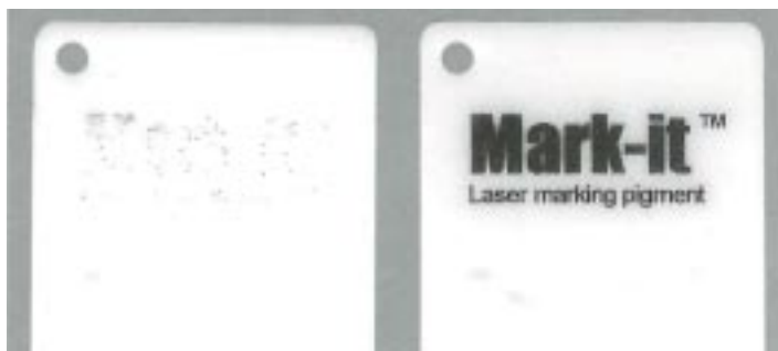
Figure 5. YAG laser marked HDPE, 0.2% TiO 2 (left) and with 0.1% Mark-it (right).
